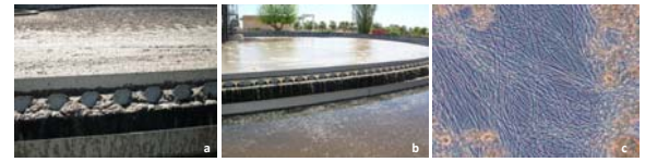
Figure 1. Activated sludge separation problems. (a) Foaming. (b) Bulking. (c) Type 021N. Phase contrast, 1000x.
